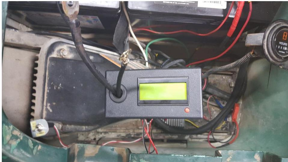
Figure 3 – BatteryAssure Sensor with the charging circuit conductor threaded through
