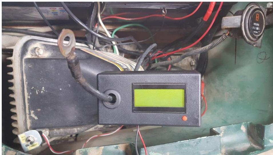
Figure 2 – BatteryAssure with the Primary drive/controller conductor threaded through
