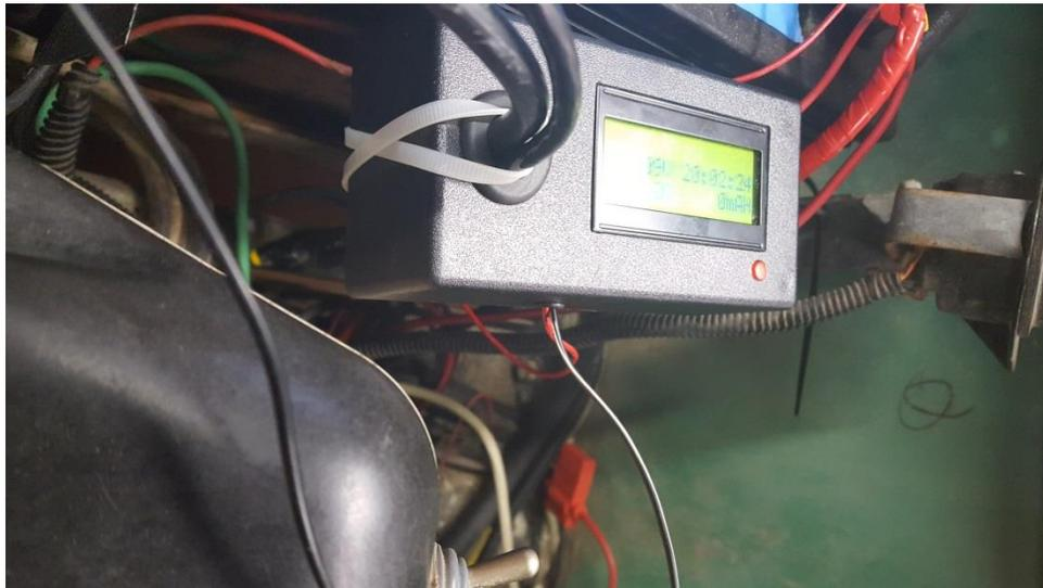
Figure 5 – Using a cable tie to secure the Sensor
