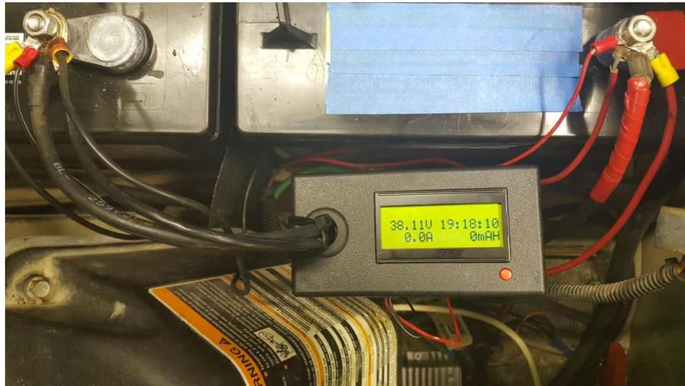
Figure 4 – BatteryAssure Sensor installation complete
